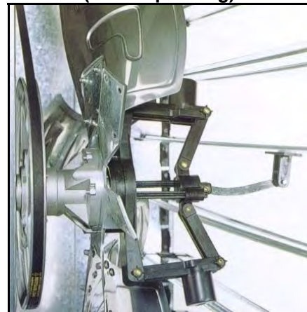
Centrifugal shutter system (fan is operating)
